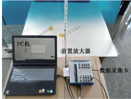
(a) 铝板落球冲击实验 (a) Impact test on aluminum plate
