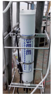
(c) 温盐深仪系统 (c) CTD (conductivity, temperature, depth) system
