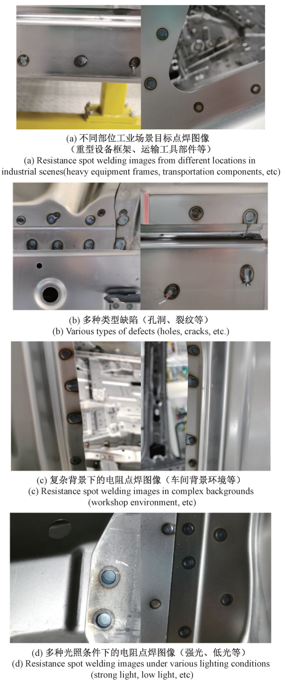
图 6 不同工业场景的电阻点焊 Fig. 6 Resistance spot welding images from different industrial scenarios
