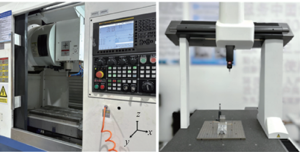
图 6 立式加工中心和加工变形测量设备 Fig. 6 Vertical machining center and machining deformation measurement equipment
