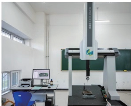
图 12 Explorer06.10.06 型三坐标测量机 Fig. 12 Explorer06.10.06 type coordinate measuring machine (CMM)
